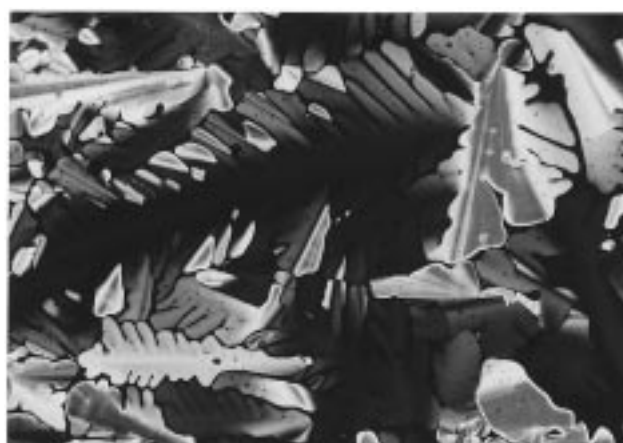
Figure 1. Texture of 2 under a polarizing microscope at 82 °C obtained after cooling from the isotropic phase to the given temperature.
